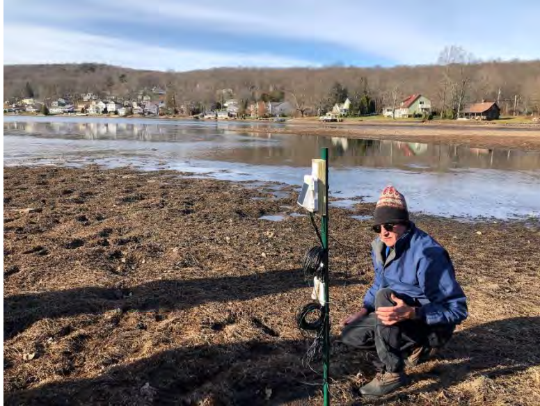
Figure 14. Monitoring sediment temperature and moisture during a deep winter drawdown of Lake Beseck, CT in 2019.
